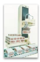
KuehnOptPal generates a valid packing sequence for robots (SCARA robots like above). Thereby not only the robot positions are calculated, also information for controlling the gripper is generated. Multiple vacuum grippers are supported.
